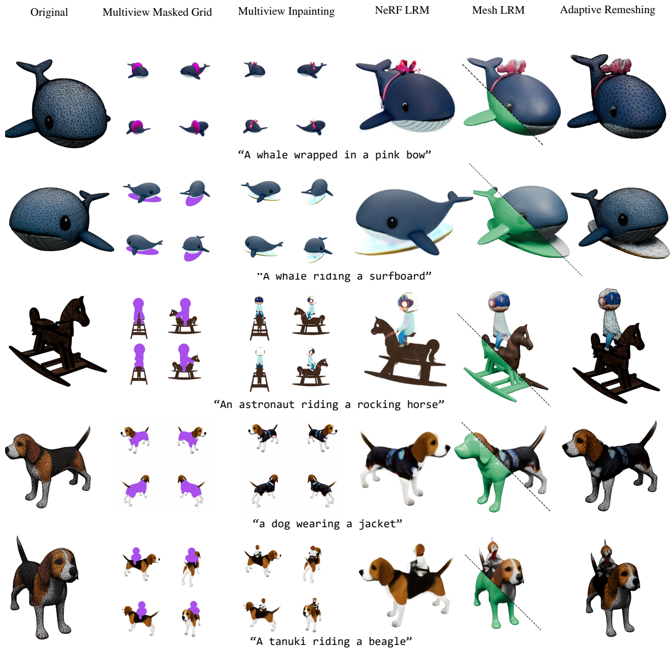
Figure 3. Gallery of results 1/3. From left to right, we show the original mesh ( column 1 ), the projected mask into four views ( column 2 ), input to Instant3dit to generate a multiview inpainted image ( column 3 ), reconstructed with NeRF-LRM ( column 4 ), and Mesh-LRM ( column 5 ), and finally, we show the adaptive remeshing results, for which we use the output of MeshLRM in a lightweight optimization that only allows part of the mesh to be modified, while retaining all pre-existing attributes (triangulation, UVs etc.) ( column 6 ).
